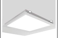
Connect cable from the solar collector. Fold one side spring clips located on the LED panel first and then do the same for the other side
